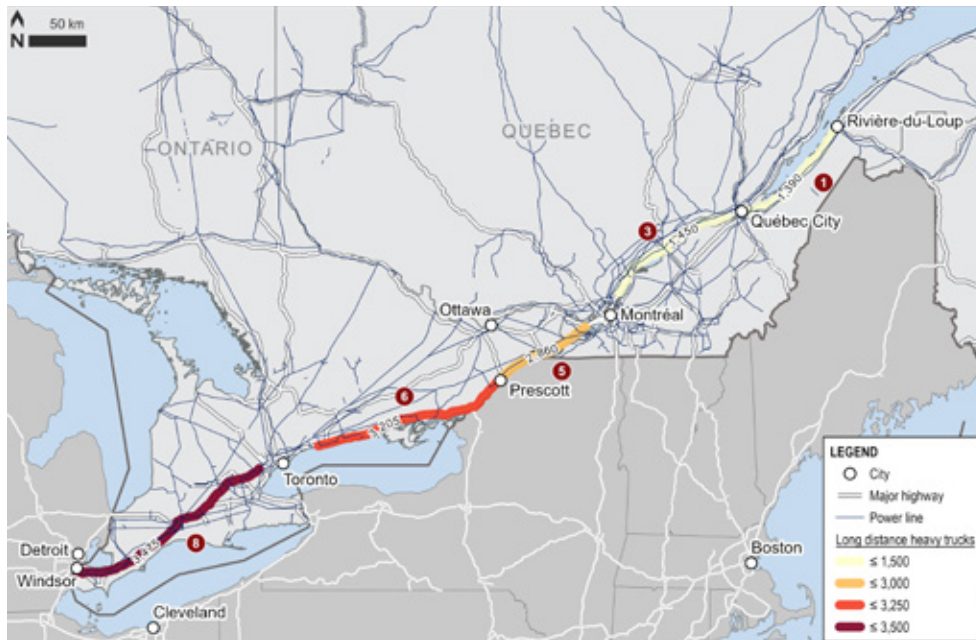
FIGURE 4. LONG DISTANCE HEAVY TRUCK VOLUME ON EACH SEGMENT OF THE STUDY CORRIDOR
