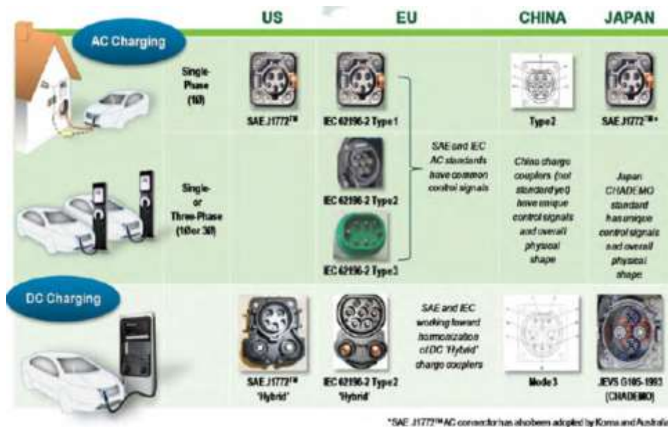
Figure 3: Conductive EV Charging Couplers
